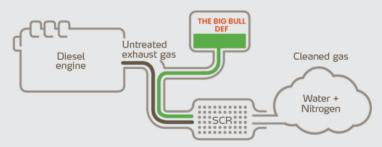
DEF can reduce the amount of Nitric Oxides in the emission can be reduced by 85%. DEF meets all BS6, BS4 objectives.
